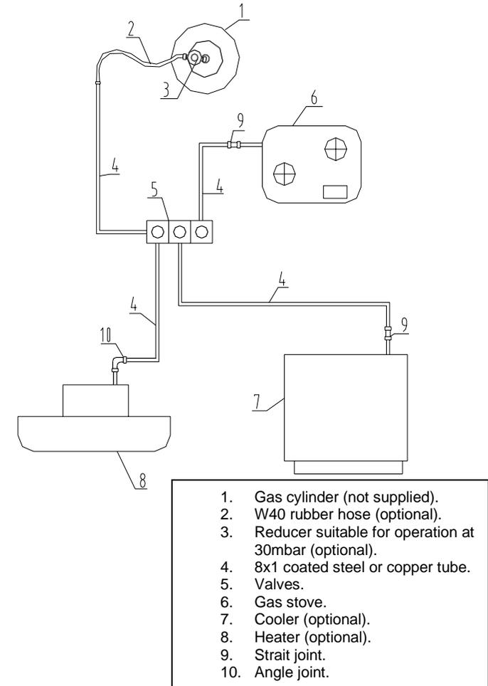
Fig. 8. Gas installation diagram.
