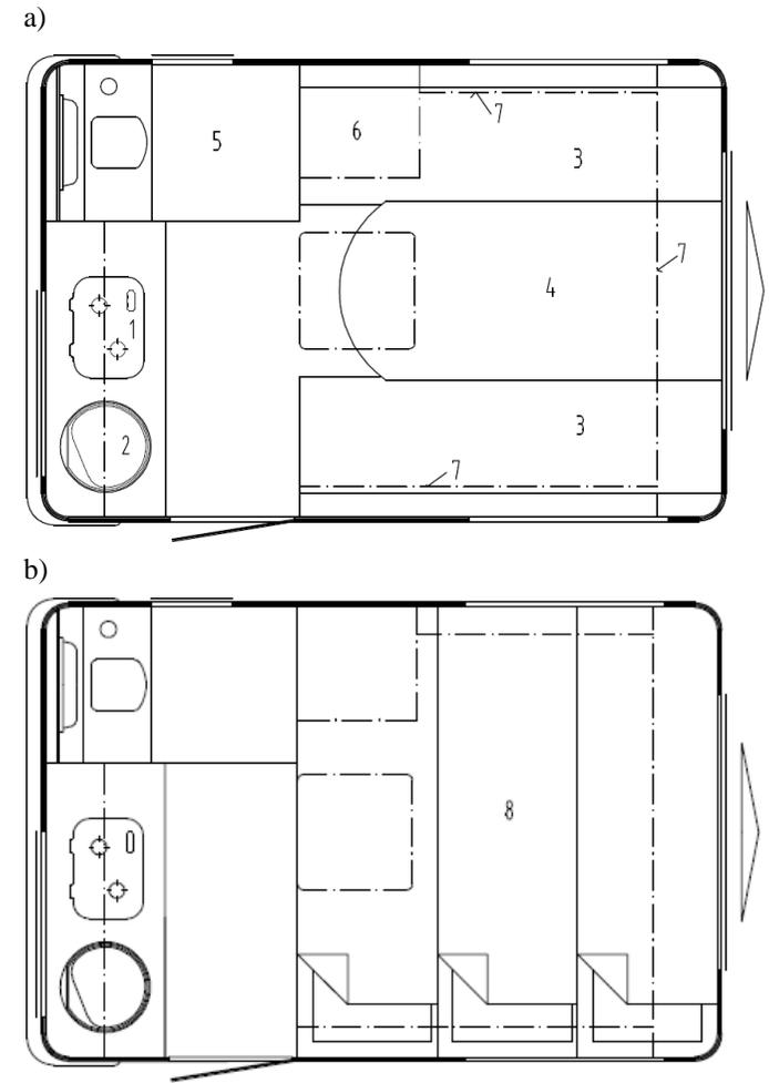
Fig. 5 Day layout (a) and night layout (b) of the N126ntl caravan (1 - gas stove, 2 - sink, 3 - front sofa, 4 - long table, 5 - bathroom, 6 - wardrobe, 7 - hanging cupboards, 8 - sleeping spot of 193x185 cm).
