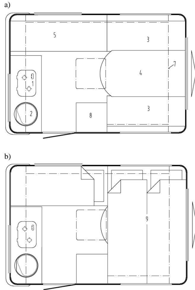
Fig. 4 Day layout (a) and night layout (b) of the N126nl caravan (1 - gas stove, 2 - sink, 3 - front sofa, 4 - long table, 5 - back sofa, 7 - hanging cupboards, 8 - side closet, 9 - sleeping spot of 130x193 cm).
